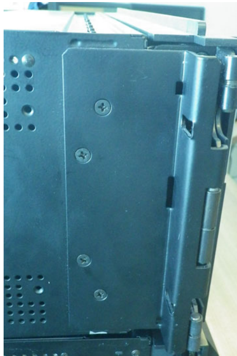
Figure 10-18: Unscrew standard front panel mounting bracket on left side
