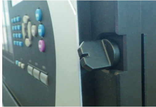
Figure 10-13: Lift latch on standard front panel to open
