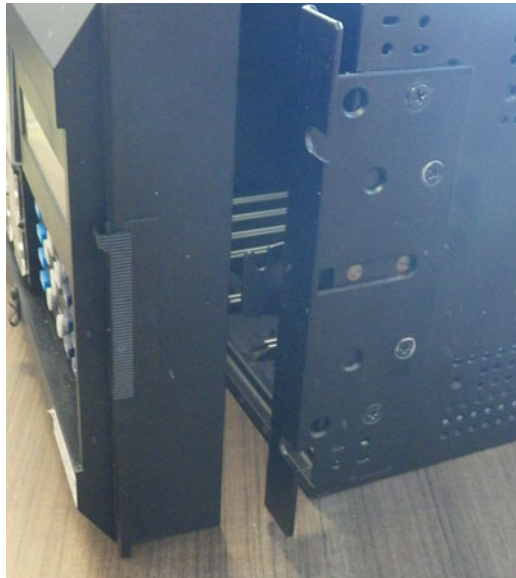
Figure 10-15: Remove standard front panel mounting bracket on right side
