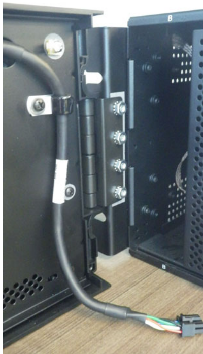
Figure 10-21: Attach to left mounting bracket inside relay
