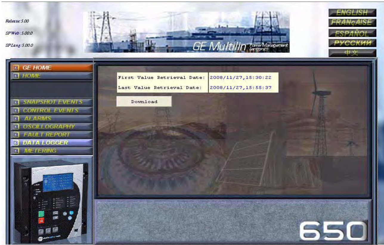
Figure 4-43: Data logger screen
