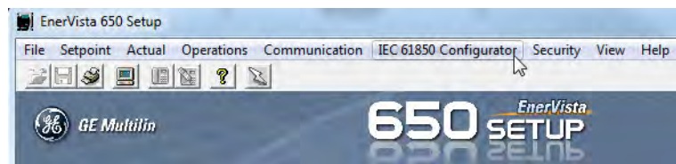
Figure 7-5: IEC61850 configurator menu location
