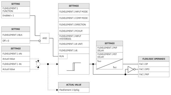
Figure 5-66: FlexElement logic
