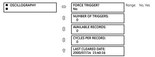
This menu allows the user to view the number of triggers involved and number of oscillography traces available. The cycles per record value is calculated to account for the fixed amount of data storage for oscillography. See the Oscillography section of chapter 5 for details.
