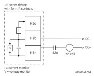
Assume the output contact H1 is a trip contact. Using the contact output settings, this output is given an ID name; for example, "Cont Op 1." Assume a 52a breaker auxiliary contact is connected to contact input H7a to monitor breaker status. Using the contact input settings, this input is given an ID name, for example, "Cont Ip 1," and is set "On" when the breaker is closed. The settings to use digital element 1 to monitor the breaker trip circuit are indicated (EnerVista example shown).
