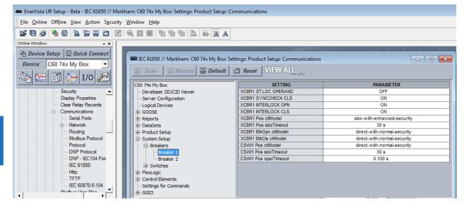
Figure 5-9: IEC 61850 protocol panel in EnerVista software
