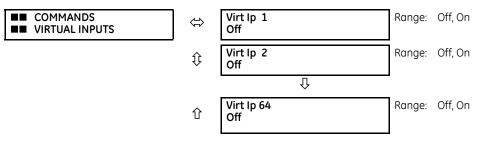
The states of up to 64 virtual inputs are changed here. The first line of the display indicates the ID of the virtual input. The second line indicates the current or selected status of the virtual input. This status is a state off (logic 0) or on (logic 1).
