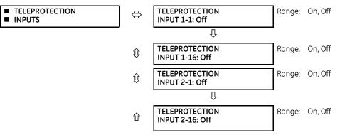
The present state of teleprotection inputs from communication channels 1 and 2 are shown here. The state displayed is that of corresponding remote output unless the channel is declared failed.
