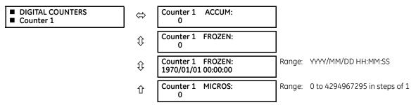
The present status of the eight digital counters displays here. The status of each counter, with the user-defined counter name, includes the accumulated and frozen counts (the count units label also appears). Also included, is the date and time stamp for the frozen count. The **COUNTER 1 MICROS** value refers to the microsecond portion of the time stamp.
