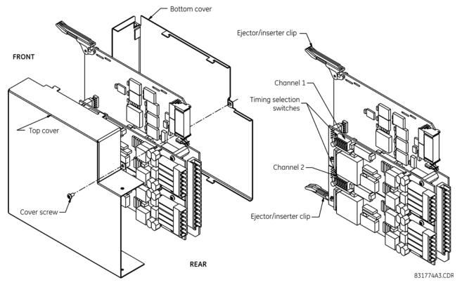
Figure 3-51: C37.94SM timing selection switch setting
