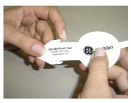
Bend the tab at the center of the tool tail as shown.
