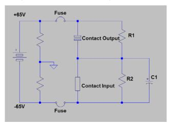
Figure 3-16: Contact input connected to a contact output with resistor (R2) across the input
