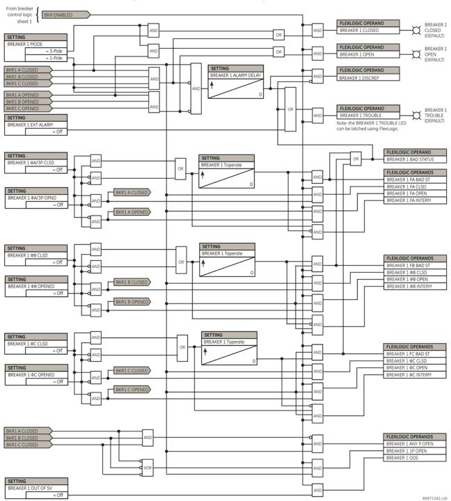
Figure 5-56: Dual breaker control logic (Sheet 2 of 2)
