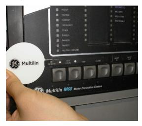
3. Remove the tool and attached user-programmable pushbutton label.
