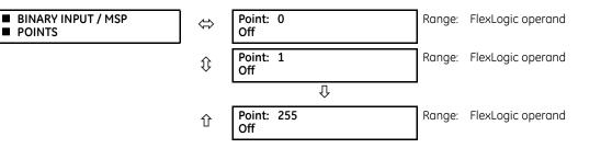
Up to 256 binary input points can be configured for the DNP or IEC 60870-5-104 protocols. The points are configured by assigning an appropriate FlexLogic operand. See the Introduction to FlexLogic section in this chapter for the range of assignable operands.
