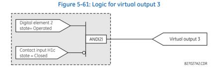
3. Prepare a logic diagram for virtual output 4, replacing the logic ahead of virtual output 3 with a symbol identified as virtual output 3, shown as follows.
