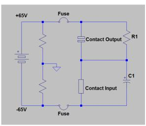
The presence of the impedance path (R1) across the contact output allows the stray (distributed) capacitance to charge as shown, thus developing a voltage across the contact input enough to momentarily operate the input while the capacitance discharges in the presence of DC ground on the positive terminal of the battery.
