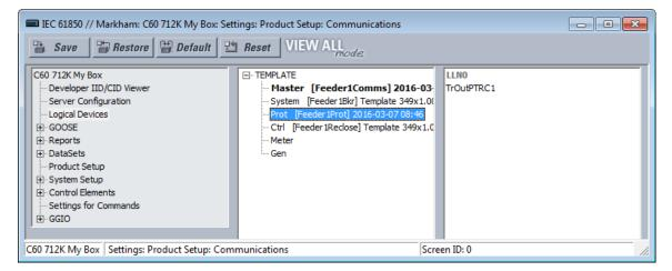
Right-clicking a logical device displays the menu that allows insertion of a new logical device immediately below the selected one, deletion of the selected logical device, or editing the selected logical device's parameters. The insert option is disabled and grayed-out if there are already 16 logical devices instantiated. The delete option is disabled and grayed-out if the selected logical device is Master or it contains any logical nodes other than LLNO.
