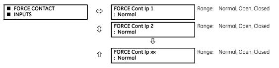
The force contact inputs feature provides a method of performing checks on the function of all contact inputs.
