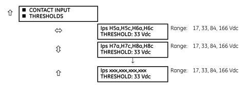
A contact inputs and outputs are digital signals associated with connections to hard-wired contacts. Wet and dry contacts are supported.
