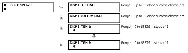
Any existing system display can be automatically copied into an available user display by selecting the existing display and pressing the **ENTER** key. The display then prompts with ADD TO USER DISPLAY LIST? After selecting "Yes," a message indicates that the selected display has been added to the user display list. When this type of entry occurs, the sub-menus are automatically configured with the proper content—this content can be edited subsequently.
