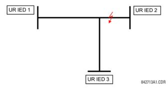
A permissive pilot-aided scheme can be implemented in a two-ring configuration, shown as follows (IEDs 1 and 2 constitute a first ring, while IEDs 2 and 3 constitute a second ring).
