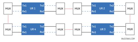
The interconnection for dual-channel type 7 communications modules is shown as follows. Two-channel modules allow for a redundant ring configuration. That is, two rings can be created to provide an additional independent data path. The required connections are: UR1-Tx1 to UR2-Rx1, UR2-Tx1 to UR3-Rx1, UR3-Tx1 to UR4-Rx1, and UR4-Tx1 to UR1-Rx1 for the first ring; and UR1-Tx2 to UR4-Rx2, UR4-Tx2 to UR3-Rx2, UR3-Tx2 to UR2-Rx2, and UR2-Tx2 to UR1-Rx2 for the second ring.
