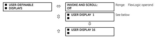
This menu provides a mechanism for manually creating up to 16 user-defined information displays in a convenient viewing sequence in the **USER DISPLAY** menu (between the **TARGETS** and **ACTUAL VALUES** top-level menus). The sub-menus facilitate text entry and Modbus register data pointer options for defining the user display content.
