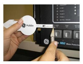
2. Slide the label tool under the user-programmable pushbutton label until the tabs snap out as shown. This attaches the label tool to the user-programmable pushbutton label.
