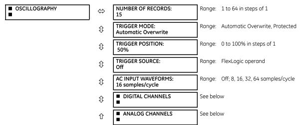
Oscillography records contain waveforms captured at the sampling rate as well as other relay data at the point of trigger. Oscillography records are triggered by a programmable FlexLogic operand. Multiple oscillography records can be captured simultaneously.
