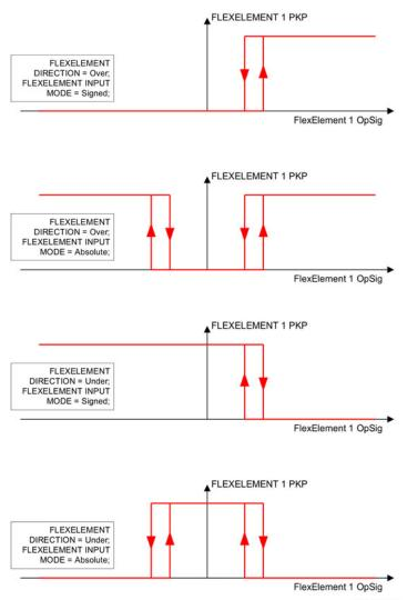
Figure 5-68: FlexElement input mode setting
