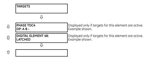
A target enables the EnerVista UR Setup software to monitor automatically and display the status of any active target messages of all the devices inserted into that site.
