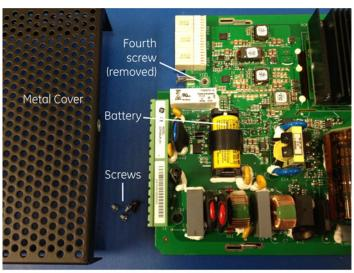
Figure 8-12: Battery location on SH/SL power supply module
