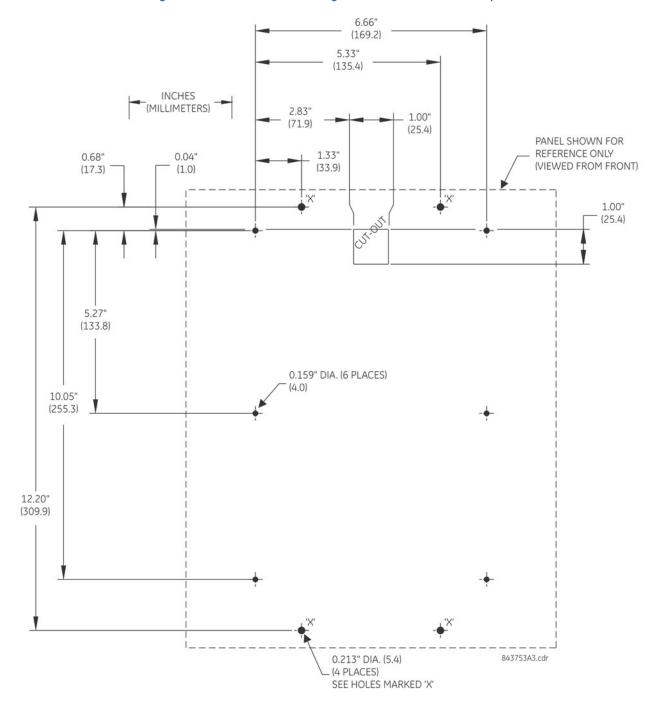
Figure 3-7: Vertical side-mounting rear dimensions (standard panel)
