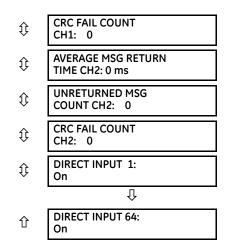
The **AVERAGE MSG RETURN TIME** is the time taken for direct output messages to return to the sender in a direct input/output ring configuration (this value is not applicable for non-ring configurations). This is a rolling average calculated for the last ten messages. There are two return times for dual-channel communications modules.
