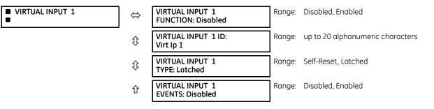
The virtual inputs and outputs are digital signals associated with UR-series internal logic signals. Virtual inputs include signals generated by the local user interface. The virtual outputs are outputs of FlexLogic equations used to customize the device. Virtual outputs can also serve as virtual inputs to FlexLogic equations.
