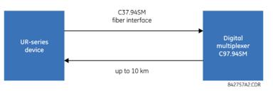
It also can be connected directly to any other UR-series relay with a C37.94SM module, as shown.
