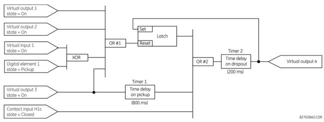
Figure 5-62: Logic for virtual output 4
