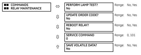
This menu contains commands for relay maintenance purposes. Commands for the lamp test and order code are activated by changing a command setting to "Yes" and pressing the **ENTER** key. The command setting then automatically reverts to "No." The service command is activated by entering a numerical code and pressing the **ENTER** key.
