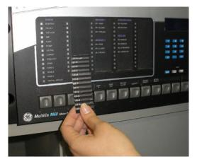
To remove the user-programmable pushbutton labels from the C30 enhanced front panel and insert the custom labels:
