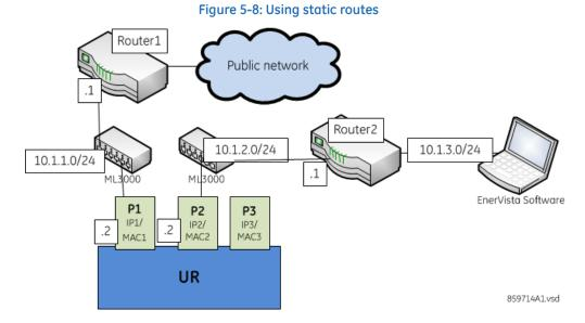
In the figure, the UR connects through the following two Ethernet ports:
