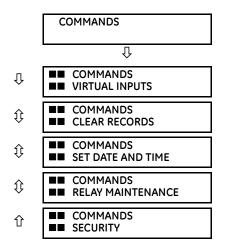
The commands menu contains relay directives intended for operations personnel. All commands can be protected from unauthorized access via the command password; see the Security section of chapter 5 for details. The following flash message appears after successfully command entry.
