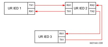
In this architecture, Devices 1 and 3 do not communicate directly. Therefore, Device 2 must act as a 'bridge'. The following settings are applied:
