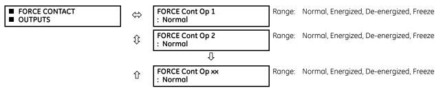
The force contact outputs feature provides a method of performing checks on the function of all contact outputs.
