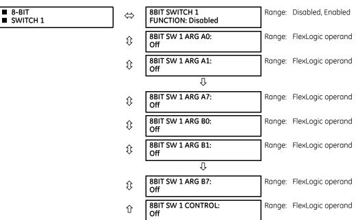
This feature allows switching between two input arguments defined by 8 bits each. The bits are specified by FlexLogic operands. The feature could be viewed as an integrated two-position switch for 8 logic signals.
