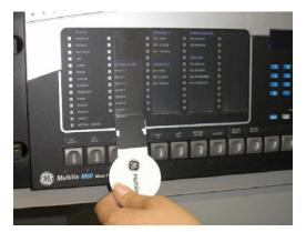
4. Slide the new LED label inside the pocket until the text is properly aligned with the LEDs, as shown.
