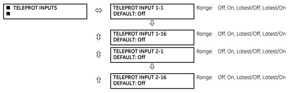
Setting the **TELEPROT INPUT** ~~ **DEFAULT** setting to "On" defaults the input to logic 1 when the channel fails. A value of "Off" defaults the input to logic 0 when the channel fails.
