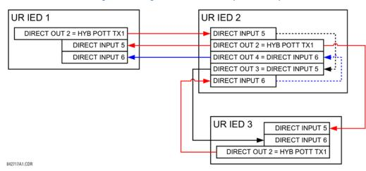
Figure 5-90: Signal flow for direct input and output
