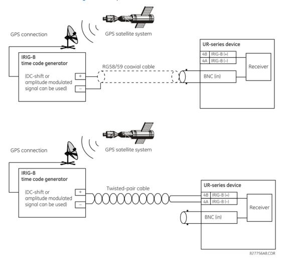
Figure 3-25: Options for the IRIG-B connection
