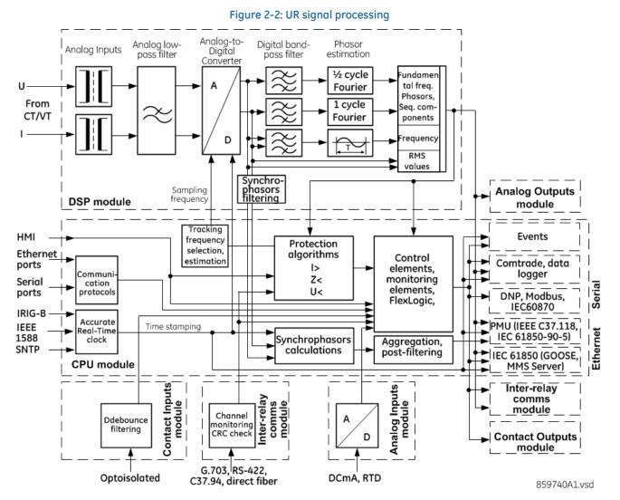
The UR samples its AC signals at 64 samples per cycle, that is, at 3840 Hz in 60 Hz systems, and 3200 Hz in 50 Hz systems. The sampling rate is dynamically adjusted to the actual system frequency by an accurate and fast frequency tracking system.
