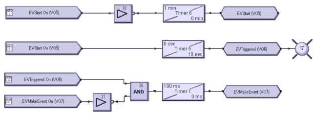
Preparation — Under **Settings > Inputs/Outputs > Virtual Outputs**, virtual output 5 is named EVStart, 6 is named EVTriggered, and 7 is named EVMakeEvent
