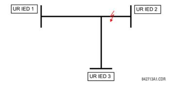
Assume the Hybrid Permissive Overreaching Transfer Trip (Hybrid POTT) scheme is applied using the architecture shown as follows. The scheme output operand HYB POTT TX1 is used to key the permission.
