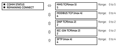
These values specify the remaining number of TCP connections still available for each protocol. The display depends on the options applicable to your device. Each time a connection is used, the remaining number of connections decrements. When released, the remaining number of connections increments. If no connection is made over the specific protocol, the number equals the maximum number available for the specific protocol.
