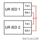
Assume that contact input 1 from UR IED 2 is to be used by UR IED 1. The following settings are applied (Direct Input 5 and bit number 12 are used, as an example).
