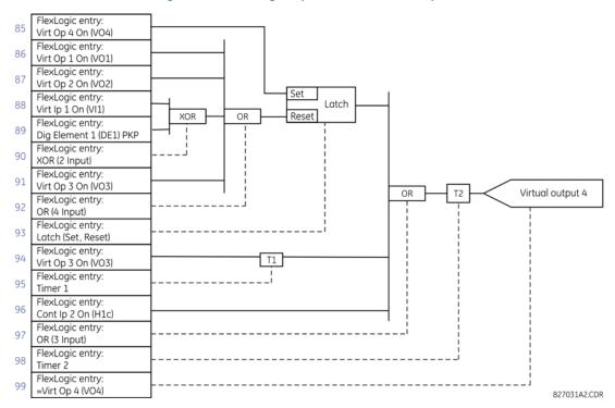
Figure 5-65: FlexLogic equation for virtual output 4
