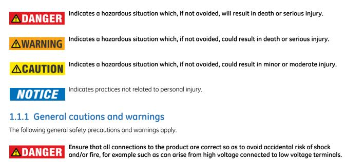
Follow the requirements of this manual, including adequate wiring size and type, terminal torque settings, voltage, current magnitudes applied, and adequate isolation/clearance in external wiring from high to low voltage circuits. Use the device only for its intended purpose and application.
