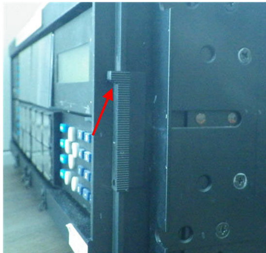
Figure 11-13: Lift latch on standard front panel to open
