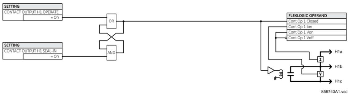
Figure 5-165: Contact input/output module type 6A contact 1 logic
