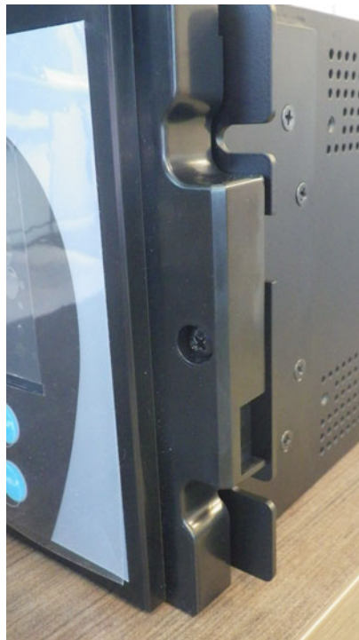
Figure 11-25: Screw to attach graphical front panel to mounting bracket
