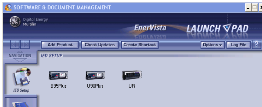
Figure 3-61: UR device added to Launchpad window
