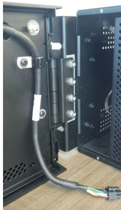
Figure 11-21: Attach to left mounting bracket inside relay
