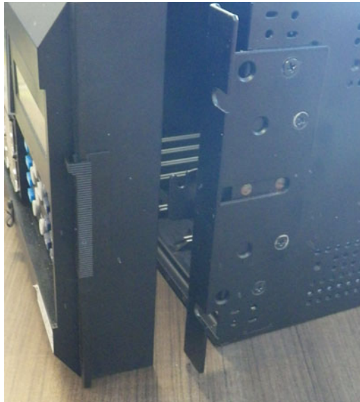
Figure 11-15: Remove standard front panel mounting bracket on right side
