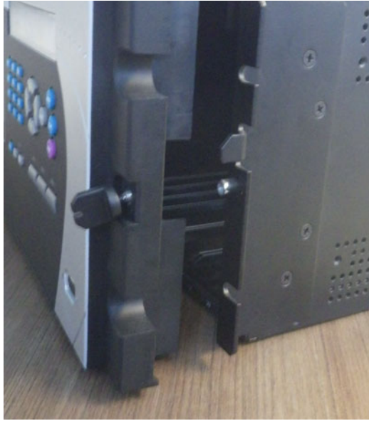
Figure 11-15: Remove standard front panel mounting bracket on right side
