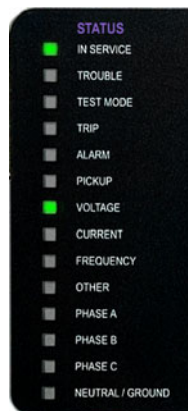
Figure 4-51: Example of LEDs on graphical front panel
