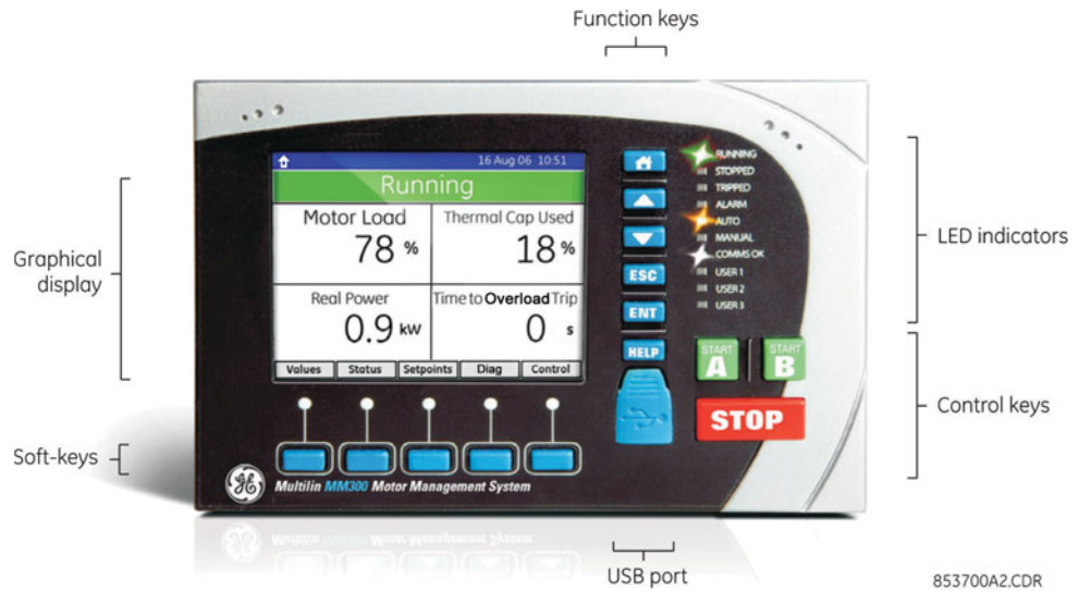
Figure 3-1: MM300 front panel with example default display
