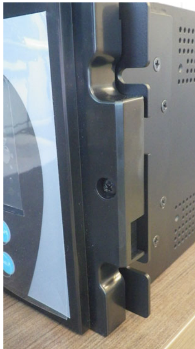
Figure 10-25: Screw to attach graphical front panel to mounting bracket
