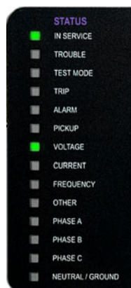
Figure 4-51: Example of LEDs on graphical front panel
