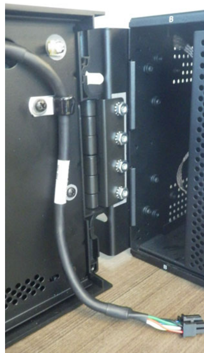
Figure 10-21: Attach to left mounting bracket inside relay
