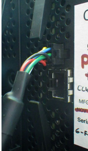
Figure 10-24: Connect graphical front panel to top connection on CPU module
