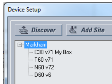
Figure 3-68: Discover button to detect UR devices in network
