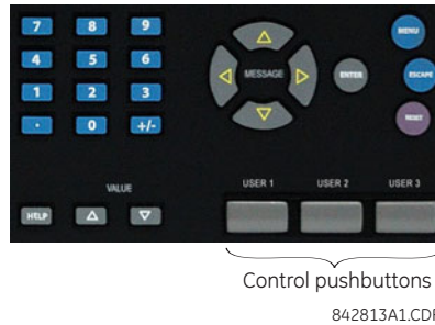
Figure 5-52: Control pushbuttons (enhanced front panel)
