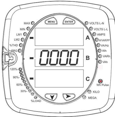
Figure 2-3: Display Showing Watt-hour Reading
