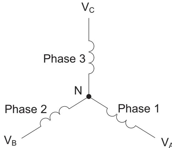
Figure B-1: Three-phase Wye Winding
