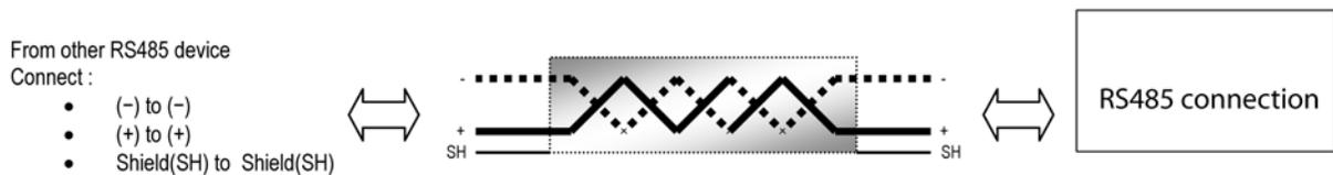
Figure 5-4: 2-wire RS485 Connection
