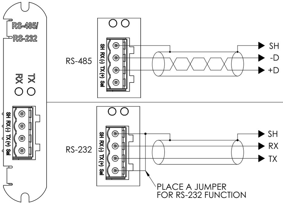
Figure 6-10: RS232/RS485 S1 Serial Communication Card
