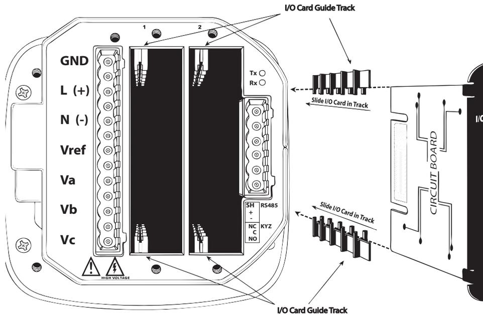
Figure 6-2: Detail of Guide Track
