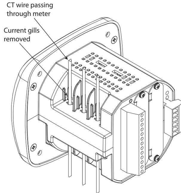
Figure 4-2: Pass Through Wire Electrical Connection
