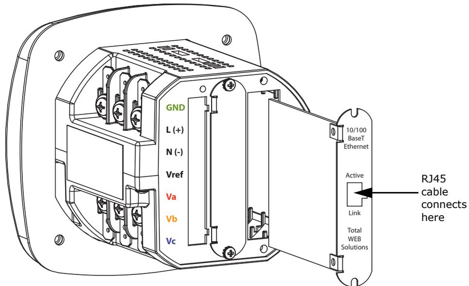
Figure 7-1: Meter with E1 Card
