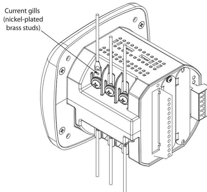
**Figure 4-1: CT Leads Terminated to Meter, #8 Screw for Lug Connection**
