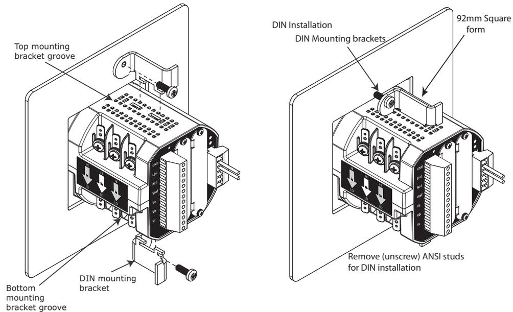
Figure 3-6: DIN Installation
