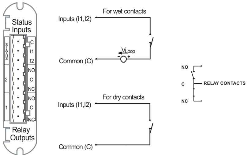
Figure 6-5: Relay Contact (2) / Status Input (2) Card
