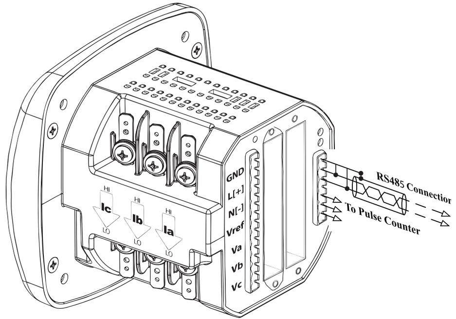
**Figure 5-2: EPM 7000P Meter Back with RS485 Communication Installation**
