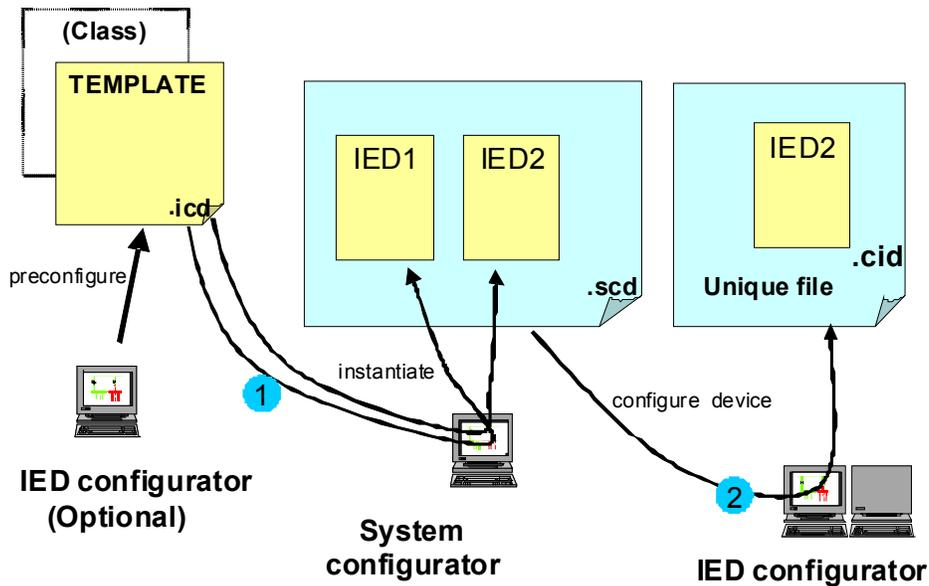
Figure 9-2: Configuration Process
