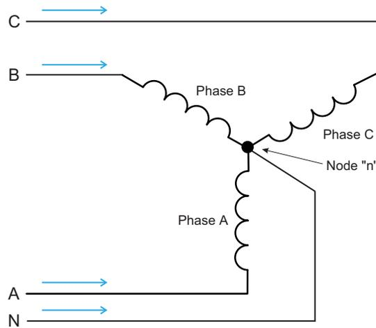
**Figure B-6: Three-Phase Wye Load Illustrating Kirchoff's Law and Blondel's Theorem**
