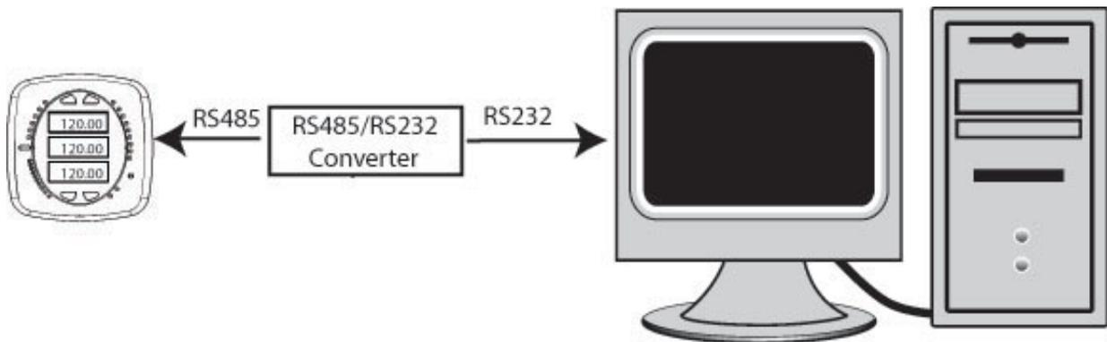
**Figure 5-3: EPM 7000P Meter Connected to a PC via RS485 bus**
