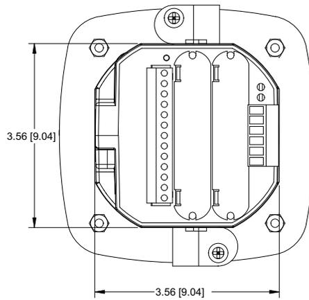
Figure 3-3: Meter Back Dimensions
