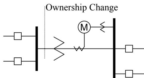
**Figure 13-1: Figure 13.1: Low Voltage Metering Installation Requiring Loss Compensation**
