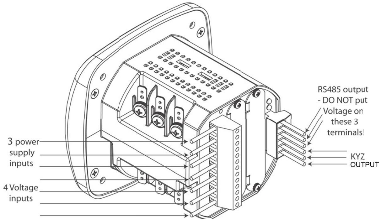
Figure 4-4: Meter Connections
