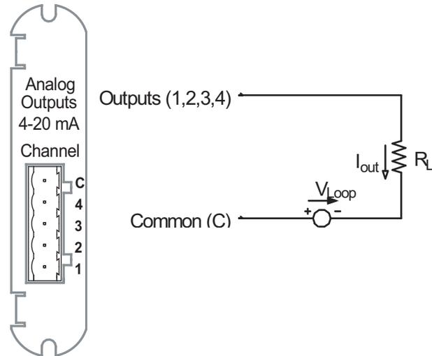
Figure 6-4: 4-Channel 4 - 20mA Output Card
