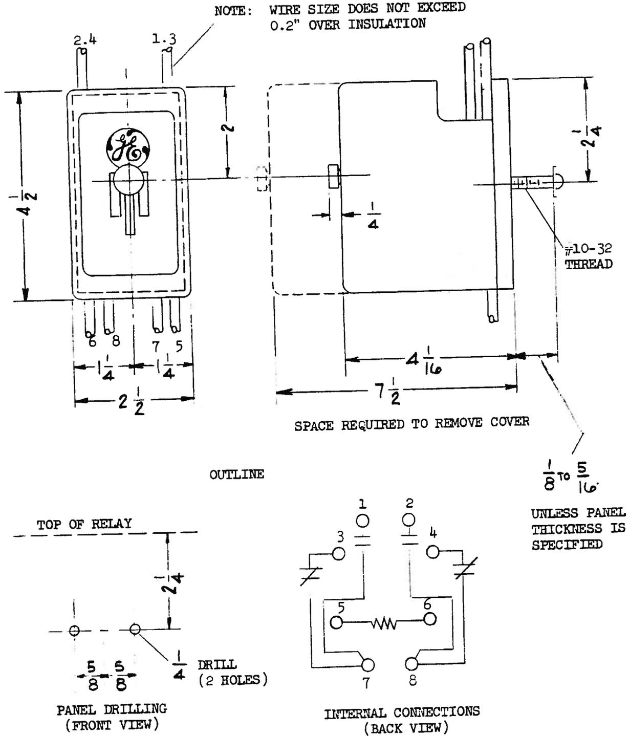
Figure 9 (0127A9568-0) Outline and Panel Drilling Dimensions for the Type HGA11T(-)A Relay
