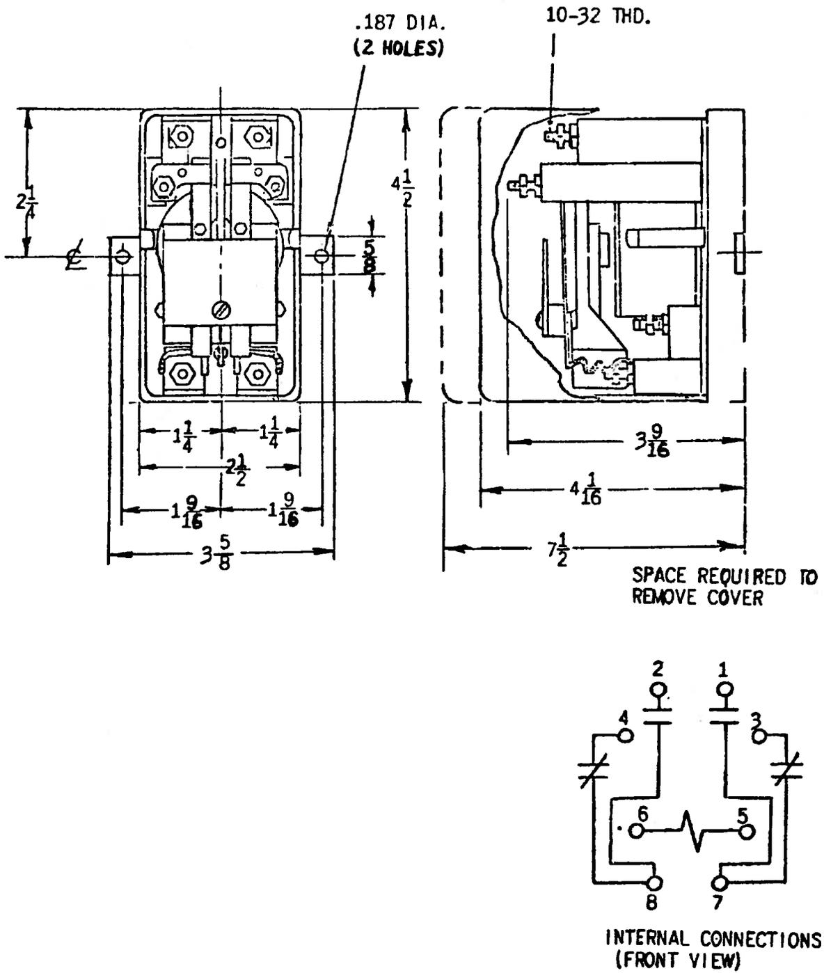
Figure 8 (0165A7757-2) Outline and Panel Drilling Dimensions for Types HGA11G, HGA11S Relays
