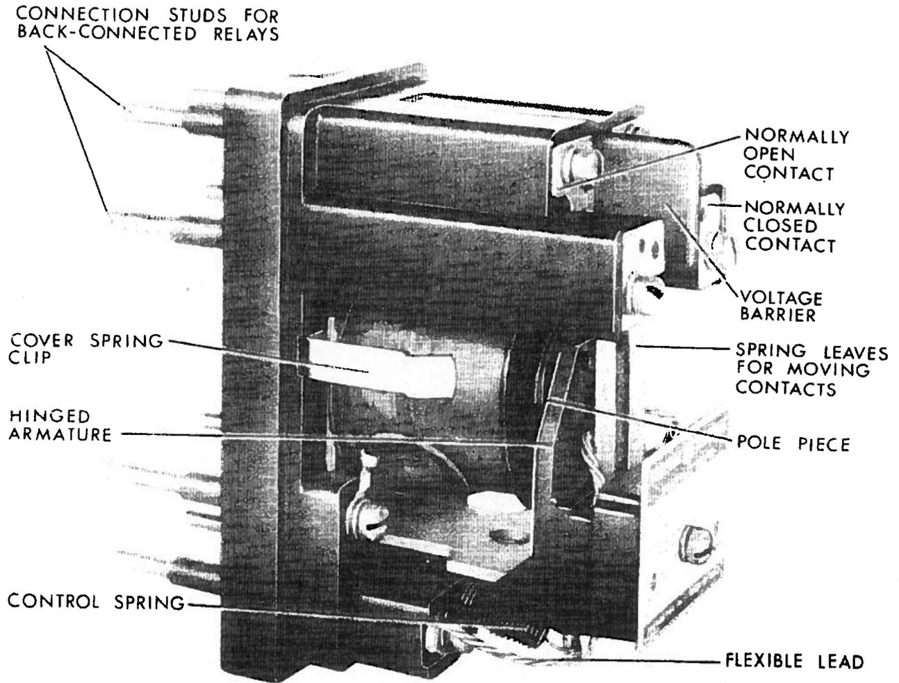
Figure 10 (8042422) Typical HGA Relay Removed from Case
