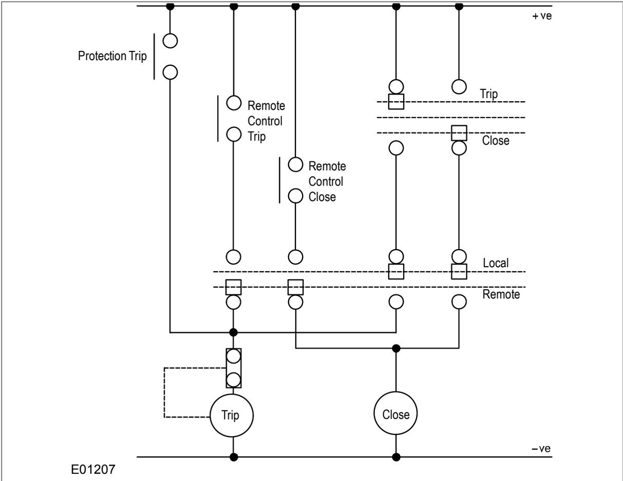
**Figure 7: Local and Remote Control of Circuit Breaker**
