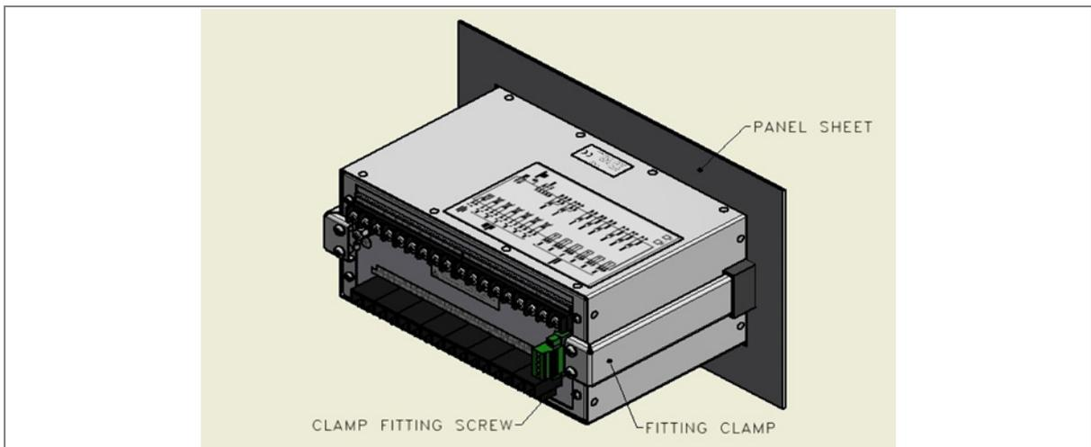
**Figure 4: Relay mounted on the panel-rear view**
