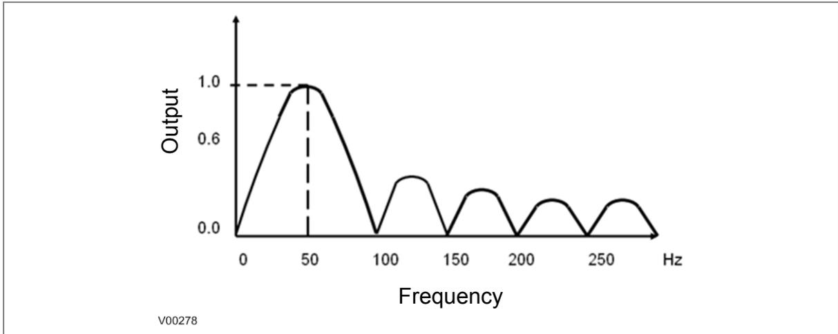
**Figure 4: Frequency response of tuned filter for 50 Hz**
