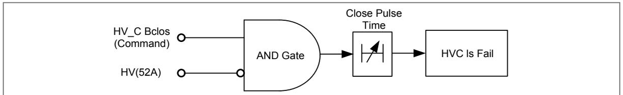
Figure 9: HV CB close fail alarm
