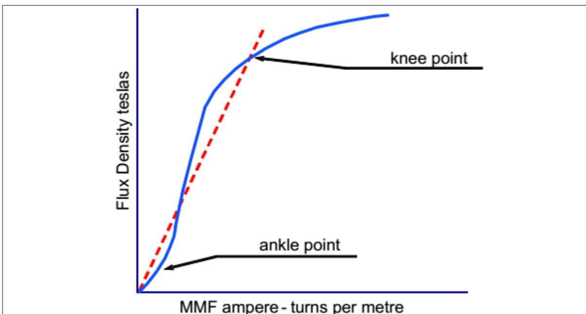
**Figure1: Exciting characteristic for a CROSS core CT**
