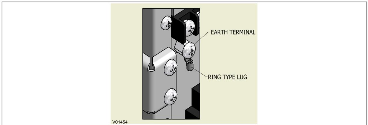
**Figure 8: Earthing terminal on the rear side of the relay**
