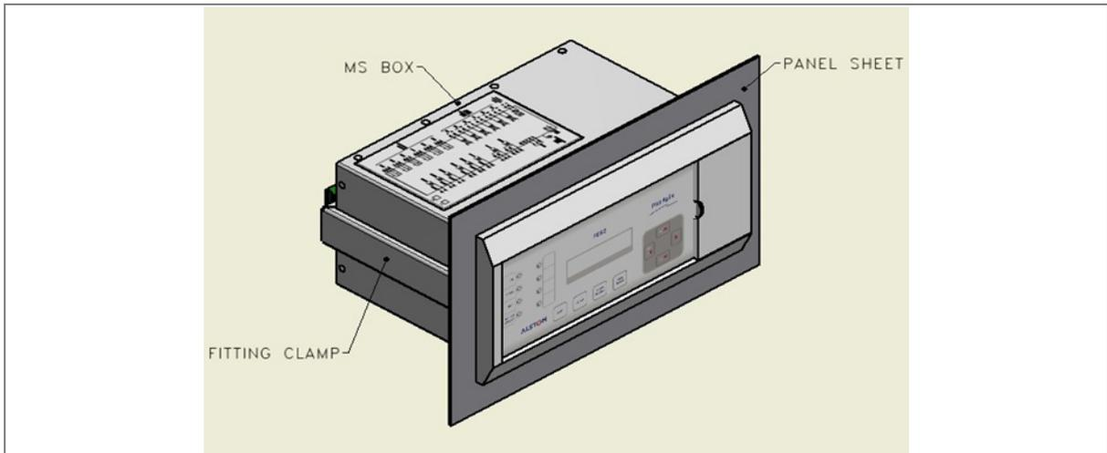
**Figure 3: Relay mounted on the panel-front view**
