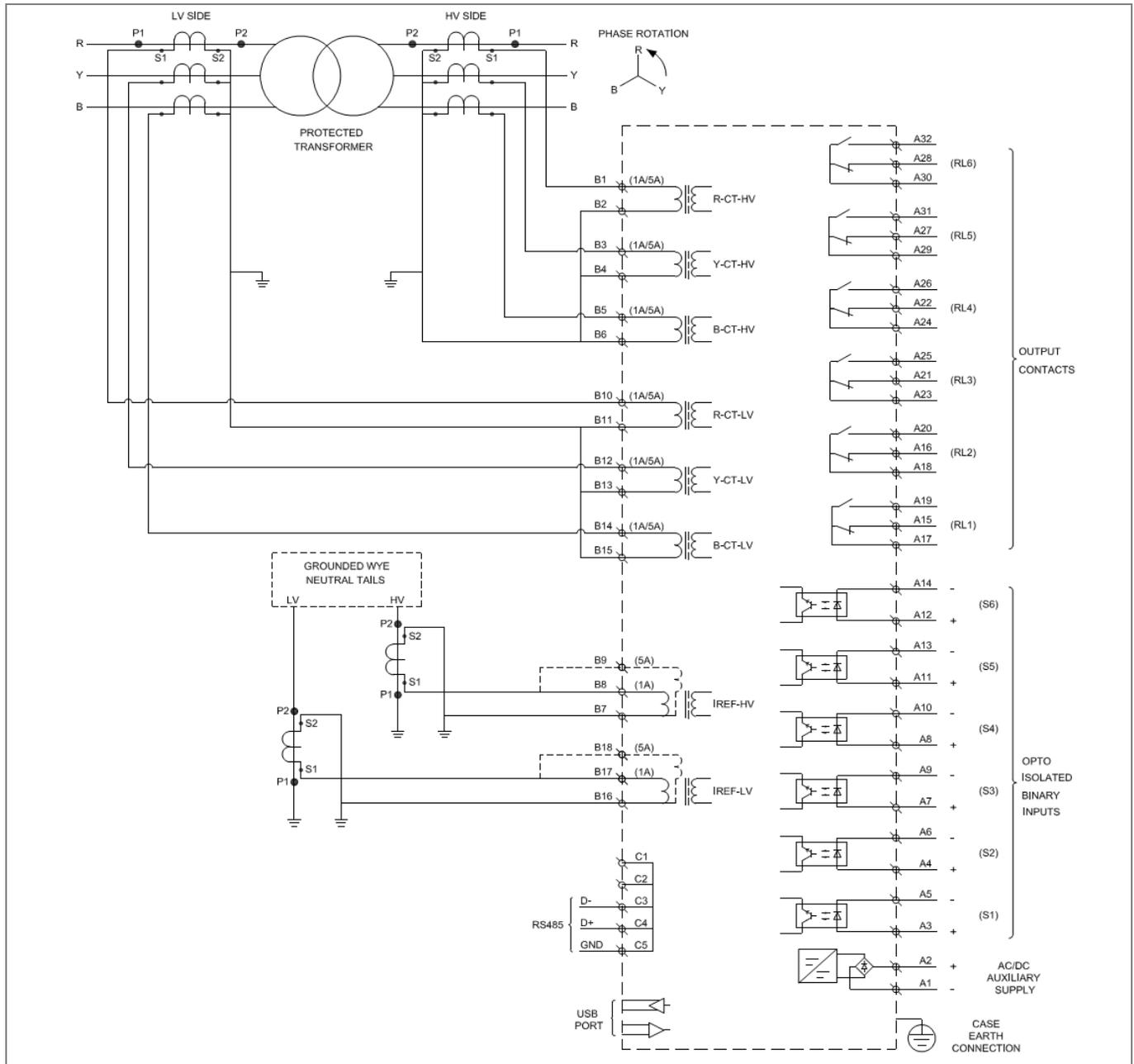
Figure 1: P652 wiring diagram
