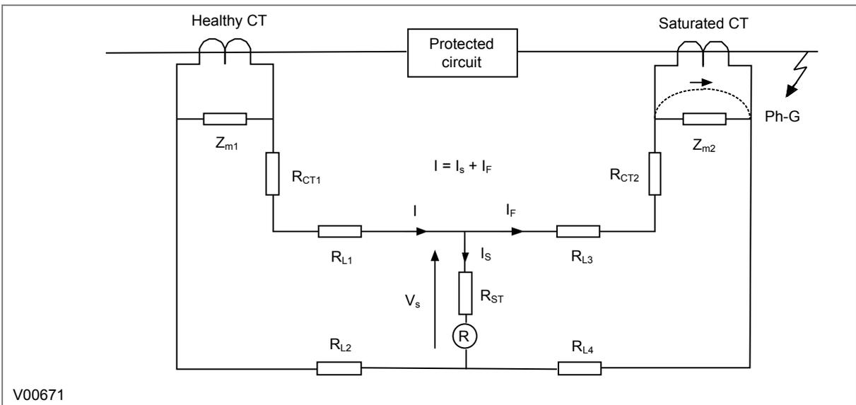
**Figure 11: High Impedance principle**
