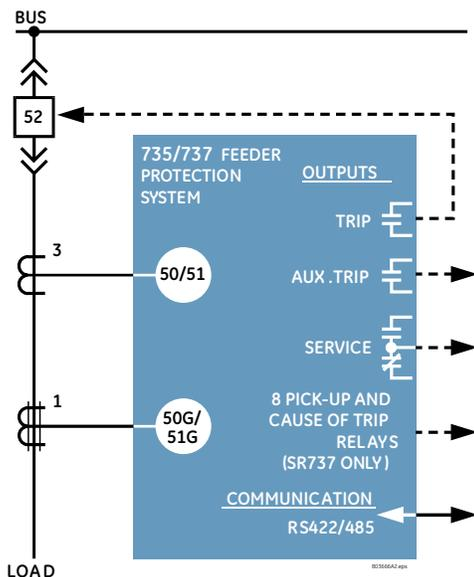
Ground level and time delay can be selected for coordination with upstream devices. The ground signal is normally derived as the residual sum of the three-phase CTs, eliminating the need for an additional ground sensor. Alternatively, for more sensitive detection, an additional core balance (zero sequence) ground sensor encircling the three-phase conductors can be used.
