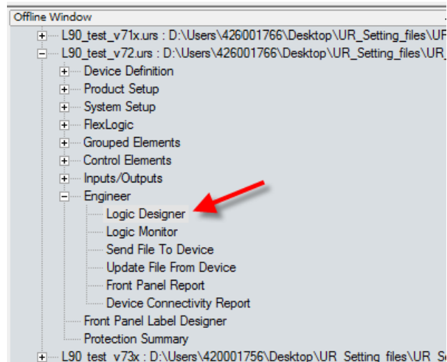
Figure 4-69: Access Engineer in the Offline Window area
