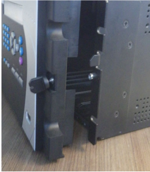
Figure 10-15: Remove basic front panel mounting bracket on right side
