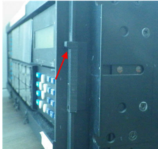
Figure 10-13: Lift latch on basic front panel to open
