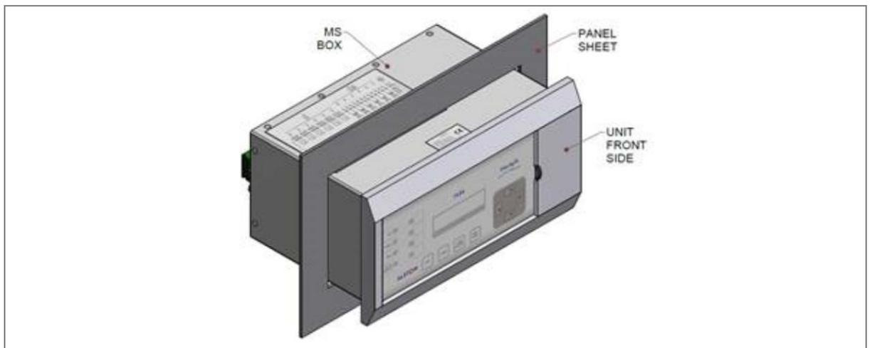
**Figure 1: Inserting relay in to the panel cutout**
