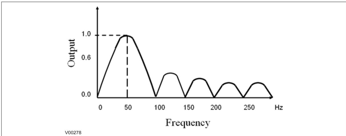
**Figure 4: Frequency response of tuned filter for 50 Hz**
