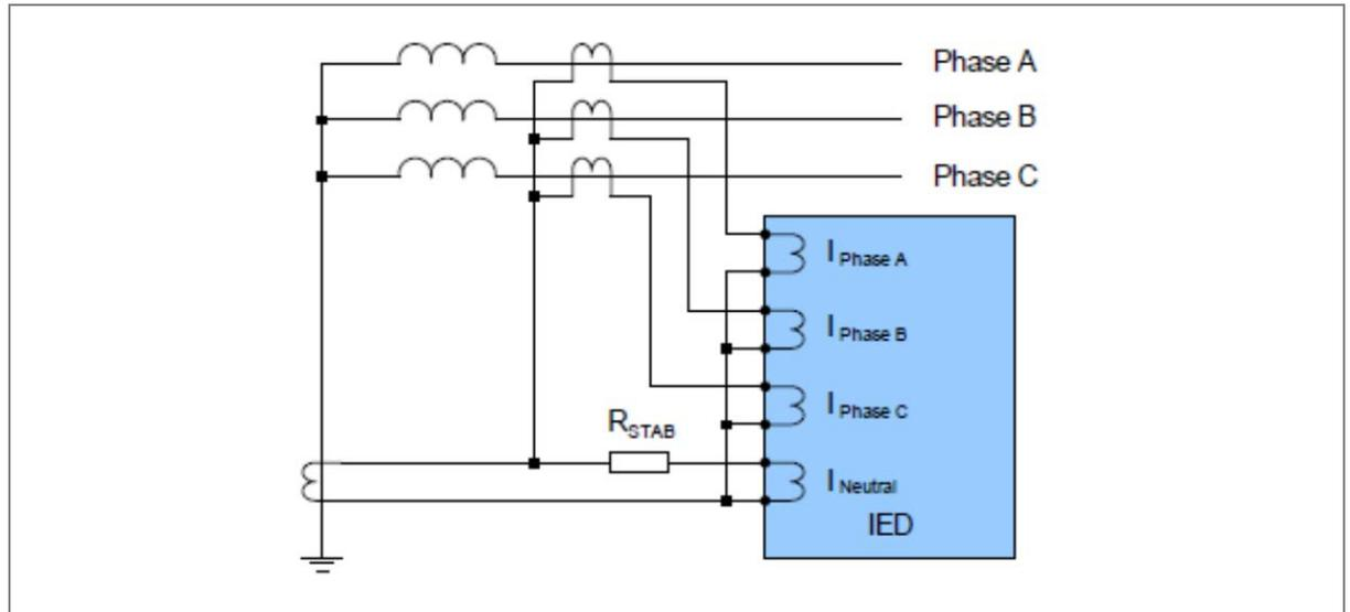
Figure 4: High Impedance REF connection
