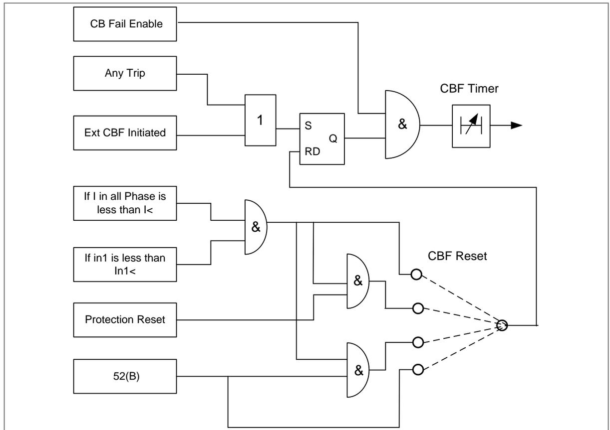
**Figure 6: CB Fail Logic**
