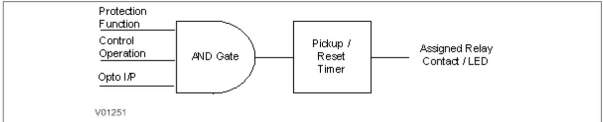
Figure 4: AND logic equation
